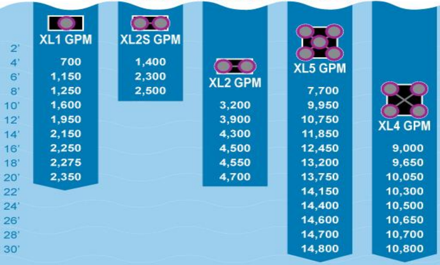
Diffuser Models Categorized by Lifting Rate GPM (Gallons Per Minute) and Water Depth
